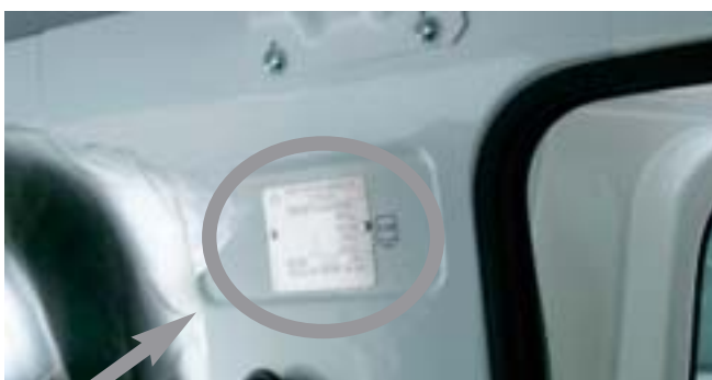
= MODEL CABSTAR = VIN PLATE LOCATION
